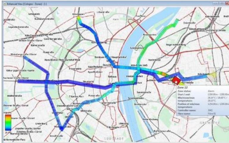
Fire detection within a tunnel
