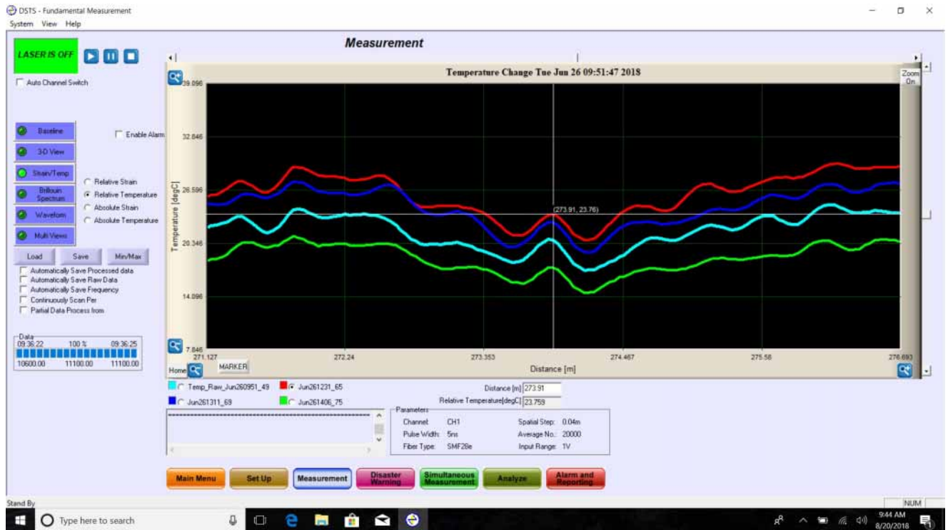
Figure 12. Temperature distributions matched well against the existing RTD readings.
