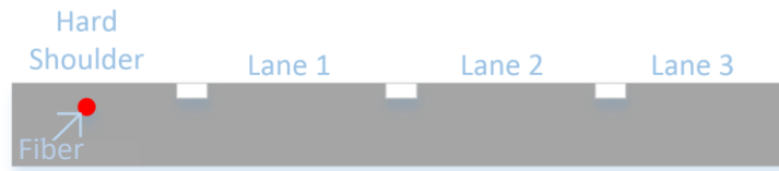
Figure 4: Example of a slot cut deployed fiber cable
