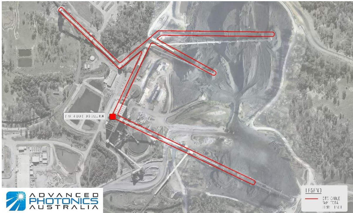
DTS cable distribution along conveyor paths
