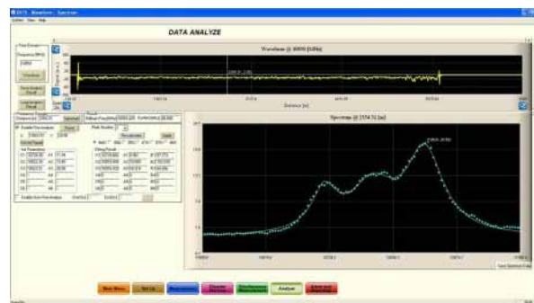
Figure 3: Brillouin spectrum with multi-peaks.
