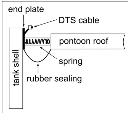
Fig. 2. Schematic of the rim seal and the mounting of the sensor cable
