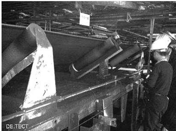
Fig. 4. View on the roller seats of a conveyor belt
