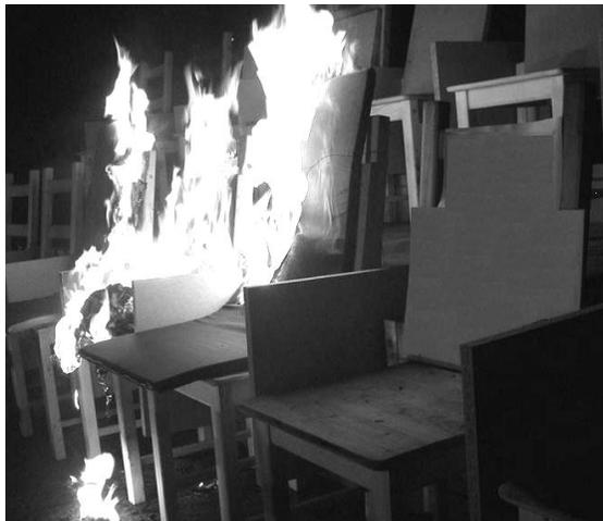
Fig. 5. Fire testing of the LHD3 response time and localisation ability
