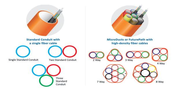
Typically, direct buried fiber cables require additional design enhancements to withstand environmental conditions, whereas a conduit can provide that environmental, tensile, and crush protection itself. The conduit itself is relatively inexpensive, so installing conduits for later use can save providers hundreds of thousands of dollars in construction costs.
